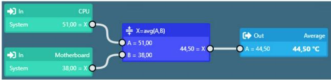
Virtual software sensors are updated once per second and re-calculated with the numbers valid in that particular moment. When using fast changing input values, extreme values can therefore either be used or ignored for the calculation. No smoothing or averaging is taking place.
